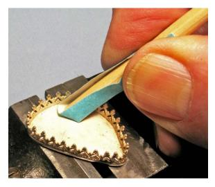
Often you'll need to sand or polish an area that's impossible to reach with even a small wheel on a flexshaft. Other times it might be the bottom of a pocket or inside bottom corner of a box that needs to be finished. One trick for these nitpicky jobs may be left over from your last Chinese dinner - a chopstick.
