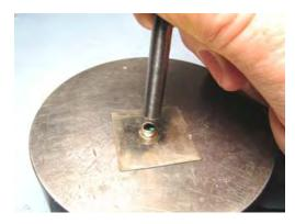
When using the tool, the first step is to capture the stone correctly. I usually work by hand and push the punch straight down over the bezel or prongs. This causes the metal to start bending over the stone. Next I inspect with a lens to be sure the stone is staying level. This is repeated until the stone is seated on its bearing and can't move anymore.
