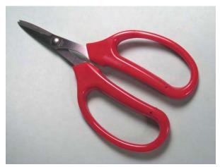
When cutting sheet metal, it's quicker and easier to use a set of shop shears as compared with using a hand saw. The cut is not as precise, but many times you don't need that. Shears will easily cut up to 24 gauge sheet, and some will cut 22 or even 20 gauge.
